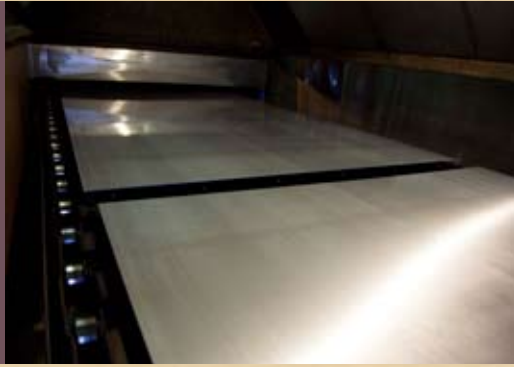
sheets enter laminating oven
