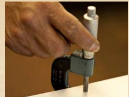
micrometer measuring blank thickness
