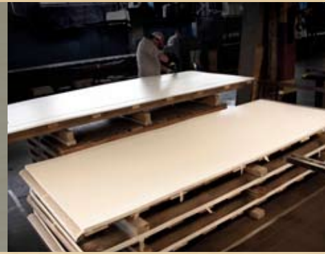
white vinyl clad sheets awaiting shearing
