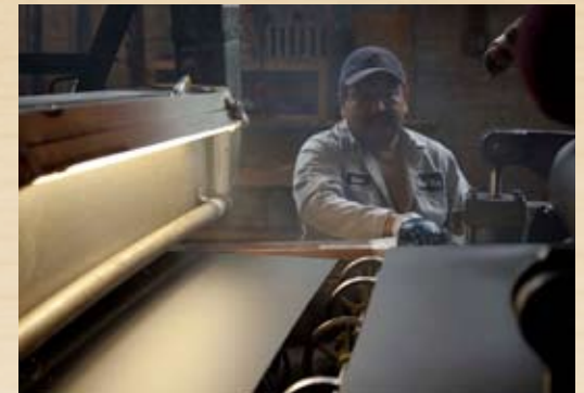
vinyl film and metal sheet are laminated
