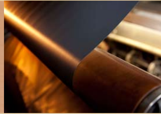
applying vinyl film upon steel
