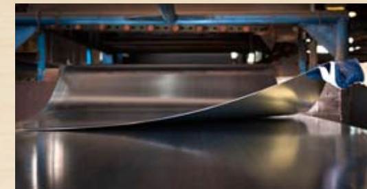
sheets exit cleaning line
