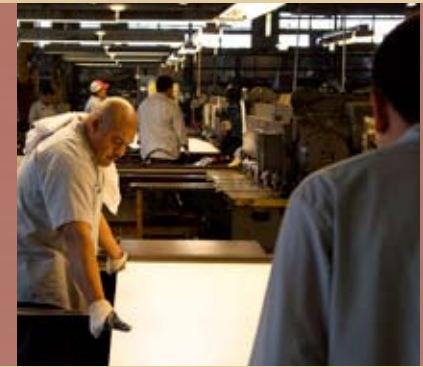
white vinyl-clad sheets at shear
